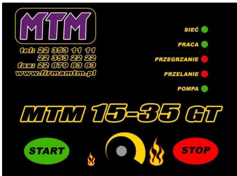
Fig. 4. The front panel of the control module of the universal oil heater type MTM15-35GT.
